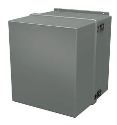
Stahlin FatBoy series enclosure, NEMA 1/3/4X/12, 18 x 16 x 17in (HxWxD), wall mount, fiberglass reinforced polyester, gray, clamshell single-door, (2) twist-lock latches, padlock hasp and staple.
