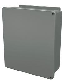
Stahlin J series enclosure, NEMA 1/3R/4X/6P/12, 16 x 14 x 6in (HxWxD), wall mount, fiberglass reinforced polyester, gray, hinged screw cover.
