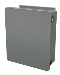
Stahlin J series enclosure, NEMA 1/3R/4X/6P/12, 16 x 14 x 6in (HxWxD), wall mount, fiberglass reinforced polyester, gray, single-door, (2) twist-lock latches.
