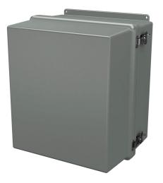
Stahlin FatBoy series enclosure, NEMA 1/3/4X/12, 16 x 14 x 12in (HxWxD), wall mount, fiberglass reinforced polyester, gray, clamshell single-door, (2) twist-lock latches, padlock hasp and staple.
