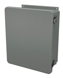
Stahlin J series enclosure, NEMA 1/3R/4X/6P/12, 14 x 12 x 6in (HxWxD), wall mount, fiberglass reinforced polyester, gray, single-door, (2) twist-lock latches.
