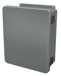
Stahlin J series enclosure, NEMA 1/3R/4X/6P/12, 12 x 10 x 5in (HxWxD), wall mount, fiberglass reinforced polyester, gray, single-door, (2) quick-release latches, padlock hasp and staple.
