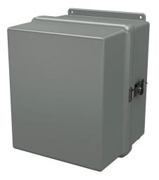
Stahlin FatBoy series enclosure, NEMA 1/3/4X/12, 12 x 10 x 10in (HxWxD), wall mount, fiberglass reinforced polyester, gray, clamshell single-door, (1) twist-lock latch, padlock hasp and staple.
