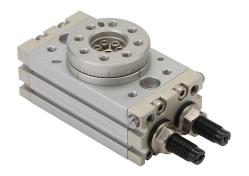
NITRA pneumatic rotary actuator, double acting, size 10, 0 to 190 degrees, shock absorbers, anodized aluminum body, M5 x 0.8 female ISO port(s).
