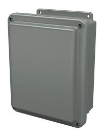
Stahlin J series enclosure, NEMA 1/3R/4X/6P/12,  $10 \times 8 \times 5$  in (HxWxD), wall mount, fiberglass reinforced polyester, gray, crowned screw cover.
