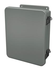
Stahlin J series enclosure, NEMA 1/3R/4X/6P/12, 10 x 8 x 4in (HxWxD), wall mount, fiberglass reinforced polyester, gray, single-door, (2) quick-release latches, padlock hasp and staple.
