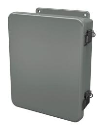
Stahlin J series enclosure, NEMA 1/3R/4X/6P/12, 10 x 8 x 4in (HxWxD), wall mount, fiberglass reinforced polyester, gray, single-door, (2) quick-release latches, padlock hasp and staple.
