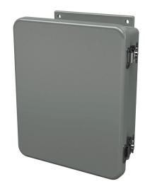
Stahlin J series enclosure, NEMA 1/3R/4X/6P/12,  $10 \times 8 \times 4$ in (HxWxD), wall mount, fiberglass reinforced polyester, gray, singledoor, (1) twist-lock latch.
