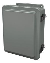
Stahlin J series enclosure, NEMA 1/3R/4X/6P/12, 10 x 8 x 5in (HxWxD), wall mount, fiberglass reinforced polyester, gray, crowned single-door, (2) quick-release latches, padlock hasp and staple.
