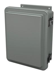
Stahlin J series enclosure, NEMA 1/3R/4X/6P/12, 10 x 8 x 5in (HxWxD), wall mount, fiberglass reinforced polyester, gray, crowned single-door, (1) twist-lock latch.
