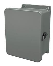
Stahlin J series enclosure, NEMA 1/3R/4X/6P/12, 10 x 8 x 6in (HxWxD), wall mount, fiberglass reinforced polyester, gray, single-door, (1) quick-release latch, padlock hasp and staple.
