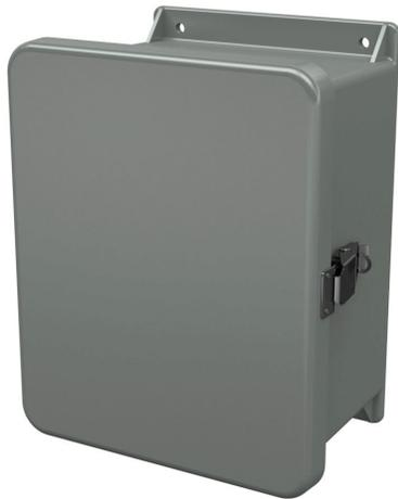
Stahlin J series enclosure, NEMA 1/3R/4X/6P/12, 10 x 8 x 6in (HxWxD), wall mount, fiberglass reinforced polyester, gray, single-door, (1) quick-release latch, padlock hasp and staple.
