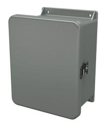
Stahlin J series enclosure, NEMA 1/3R/4X/6P/12, 10 x 8 x 6in (HxWxD), wall mount, fiberglass reinforced polyester, gray, single-door, (1) twist-lock latch.
