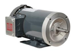
Marathon premium efficiency AC induction motor, centrifugal jet pump and inverter rated, 3hp, 3-phase, 230/460 VAC, 3600rpm, TEFC, 56HJ frame, rolled steel, C-face/rigid base mount. Drip cover and mounting hardware included.
