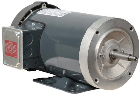
Marathon premium efficiency AC induction motor, centrifugal jet pump and inverter rated, 3hp, 3-phase, 230/460 VAC, 3600rpm, TEFC, 56HJ frame, rolled steel, C-face/rigid base mount. Drip cover and mounting hardware included.
