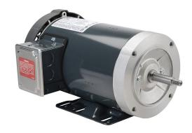
Marathon premium efficiency AC induction motor, centrifugal jet pump and inverter rated, 2hp, 3-phase, 230/460 VAC, suitable for 208 VAC at 60 Hz, 3600rpm, TEFC, NEMA 56J frame, rolled steel, C-face/rigid base mount.
