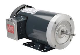
Marathon premium efficiency AC induction motor, centrifugal jet pump and inverter rated, 2hp, 3-phase, 230/460 VAC, suitable for 208 VAC at 60 Hz, 3600rpm, TEFC, 56J frame, rolled steel, C-face/rigid base mount.
