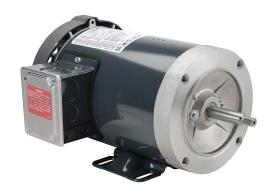
Marathon premium efficiency AC induction motor, centrifugal jet pump and inverter rated, 1-1/2hp, 3-phase, 208-230/460 VAC, 3600rpm, TEFC, 56J frame, rolled steel, C-face/rigid base mount.
