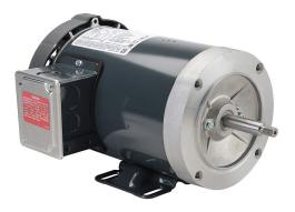
Marathon premium efficiency AC induction motor, centrifugal jet pump and inverter rated, 1-1/2hp, 3-phase, 208-230/460 VAC, 3600rpm, TEFC, NEMA 56J frame, rolled steel, C-face/rigid base mount.
