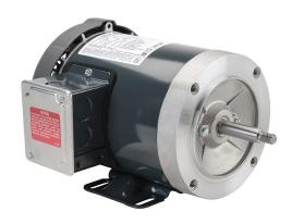
Marathon premium efficiency AC induction motor, centrifugal jet pump and inverter rated, 1hp, 3-phase, 230/460 VAC, suitable for 208 VAC at 60 Hz, 3600rpm, TEFC, NEMA 56J frame, rolled steel, C-face/rigid base mount.
