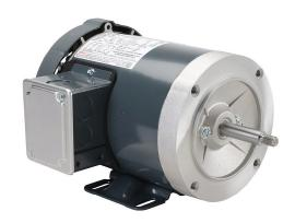
Marathon standard efficiency AC induction motor, centrifugal jet pump and inverter rated, 1/2hp, 3-phase, 208-230/460 VAC, 3600rpm, TEFC, 56J frame, rolled steel, C-face/rigid base mount.
