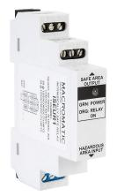
Macromatic intrinsically safe relay, 35mm DIN rail mount, fingersafe, Discrete Input: 1-point, 10 VDC input voltage, 102-132 VAC or 10-125 VDC coil voltage, Discrete Output: 1-point, relay, SPST, 5A contact rating, (1) N.O., LED indicator(s).
