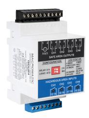
Macromatic intrinsically safe relay, 35mm DIN rail mount, fingersafe, Discrete Input: 4-point, 10 VDC input voltage, 102-132 VAC or 10-125 VDC coil voltage, Discrete Output: 4-point, relay, 4PST, 5A contact rating, (4) N.O., LED indicator(s).
