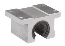
PBC IPP series single pillow block, full ball recirculating bearing, 1.88in overall length, steel, 3/4in inside diameter, aluminum housing. For use with 3/4in diameter PBC shafts.
