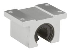
PBC IPP series single pillow block, full ball recirculating bearing, 1.75in overall length, steel, 5/8in inside diameter, aluminum housing. For use with 5/8in diameter PBC shafts.
