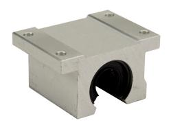
PBC IPP series single pillow block, full ball recirculating bearing, 1.5in overall length, steel, 1/2in inside diameter, aluminum housing. For use with 1/2in diameter PBC shafts.
