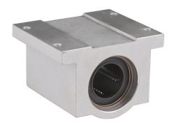
PBC IP series single pillow block, full ball recirculating bearing, 2.81in overall length, steel, 1in inside diameter, aluminum housing. For use with 1in diameter PBC shafts.
