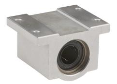
PBC IP series single pillow block, full ball recirculating bearing, 1.94in overall length, steel, 5/8in inside diameter, aluminum housing. For use with 5/8in diameter PBC shafts.
