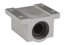
PBC IP series single pillow block, full ball recirculating bearing, 1.69in overall length, steel, 1/2in inside diameter, aluminum housing. For use with 1/2in diameter PBC shafts.
