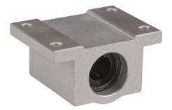
PBC IP series single pillow block, full ball recirculating bearing, 1.31in overall length, steel, 3/8in inside diameter, aluminum housing. For use with 3/8in diameter PBC shafts.
