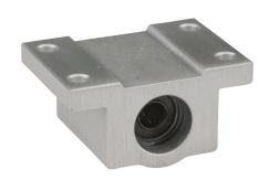
PBC IP series single pillow block, full ball recirculating bearing, 1.19in overall length, steel, 1/4in inside diameter, aluminum housing. For use with 1/4in diameter PBC shafts.
