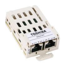
Toshiba communication module, EtherCAT CoE protocol, 2 ports, (2) Ethernet (RJ45) port(s). For use with Toshiba AS3 series AC drives.
