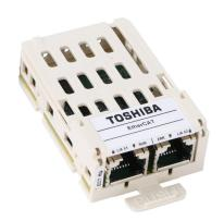
Toshiba communication module, EtherCAT Slave, 2 ports, (2) Ethernet (RJ45) port(s). For use with Toshiba AS3 series AC drives.
