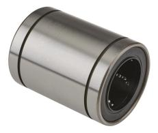
PBC IP series closed full ball recirculating bearing, steel, 1-1/4in inside diameter, 2in outside diameter, 2-5/8in overall length. For use with 1-1/4in diameter PBC shafts.
