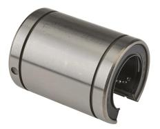
PBC IP series open full ball recirculating bearing, steel, 1-1/4in inside diameter, 2in outside diameter, 2-5/8in overall length. For use with 1-1/4in diameter PBC shafts.
