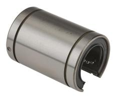
PBC IP series open full ball recirculating bearing, steel, 1in inside diameter, 1-9/16in outside diameter, 2-1/4in overall length. For use with 1in diameter PBC shafts.
