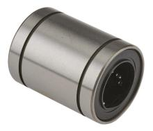
PBC IP series closed full ball recirculating bearing, steel, 3/4in inside diameter, 1-1/4in outside diameter, 1-5/8in overall length. For use with 3/4in diameter PBC shafts.
