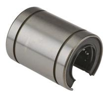
PBC IP series open full ball recirculating bearing, steel, 3/4in inside diameter, 1-1/4in outside diameter, 1-5/8in overall length. For use with 3/4in diameter PBC shafts.
