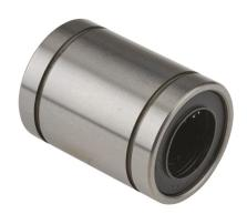
PBC IP series closed full ball recirculating bearing, steel, 5/8in inside diameter, 1-1/8in outside diameter, 1-1/2in overall length. For use with 5/8in diameter PBC shafts.
