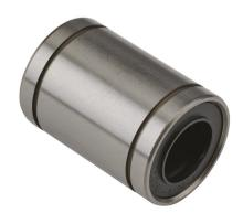
PBC IP series closed full ball recirculating bearing, steel, 1/2in inside diameter, 7/8in outside diameter, 1-1/4in overall length. For use with 1/2in diameter PBC shafts.
