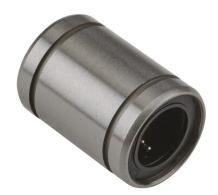
PBC IP series closed full ball recirculating bearing, steel, 3/8in inside diameter, 5/8in outside diameter, 7/8in overall length. For use with 3/8in diameter PBC shafts.
