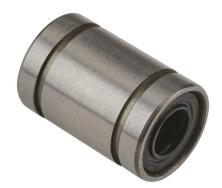
PBC IP series closed full ball recirculating bearing, steel, 1/4in inside diameter, 1/2in outside diameter, 3/4in overall length. For use with 1/4in diameter PBC shafts.
