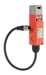
IDEM safety switch, tongue (key) interlock, slow action break before make, (2) N.C. safety output(s), plastic body, 316 stainless steel head, (1) 8-pin M12 quick-disconnect.
