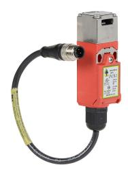
IDEM safety switch, tongue (key) interlock, slow action break before make, (1) N.C. safety output(s), plastic body, 316 stainless steel head, (1) 4-pin M12 quick-disconnect.
