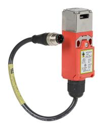
IDEM safety switch, tongue (key) interlock, slow action, (2) N.C. safety output(s), plastic body, 316 stainless steel head, (1) 4-pin M12 quick-disconnect.
