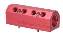
CITO Inline air, coolant, oil or water manifold, anodized aluminum, red, rectangular, 3000 psi maximum operating pressure, (4) stations, (2) 3/4in female NPT inlet(s), (8) 1/4in female NPT outlet(s), 45-deg and 135-deg orientation.
