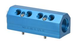
CITO Inline air, coolant, oil or water manifold, anodized aluminum, blue, rectangular, 3000 psi maximum operating pressure, (4) stations, (2) 3/4in female NPT inlet(s), (8) 1/4in female NPT outlet(s), 45-deg and 135-deg orientation.
