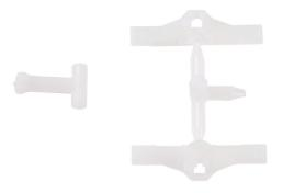
WEG Electric mechanical interlock, side mount. For use with CWBx9 to CWBx38 series contactors. Allows for mechanical connection of two contactors to prevent both from being pulled in at the same time. Adds zero to width.
