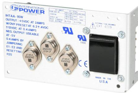
International Power regulated linear power supply, 5 VDC @ 2A/10W, 12 or 15 VDC @ 0.4A/6W and -5, -12 or -15 VDC @ 0.4A/6W, 120/240 VAC nominal input, 1-phase, open frame, aluminum housing, chassis mount, turret terminals.
