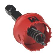
MK Morse hole saw, 7/8in (22mm), bi-metal cobalt, hardened steel backer, straight pitch, 1/8in (3.2mm) maximum cutting depth.
