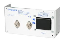
International Power regulated linear power supply, 5 VDC @ 6A/30W and 12-15 VDC @ 2.5A/30W, 120/240 VAC nominal input, 1-phase, open frame, aluminum housing, chassis mount, turret terminals.
