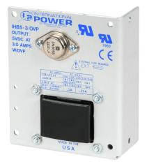
International Power regulated linear power supply, 5 VDC @ 3A/15W, 120/240 VAC nominal input, 1-phase, open frame, aluminum housing, chassis mount, turret terminals.
